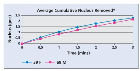
Removes approximately 2.3 grams of nuclear material in a three minute run time regardless of disc hydration.
